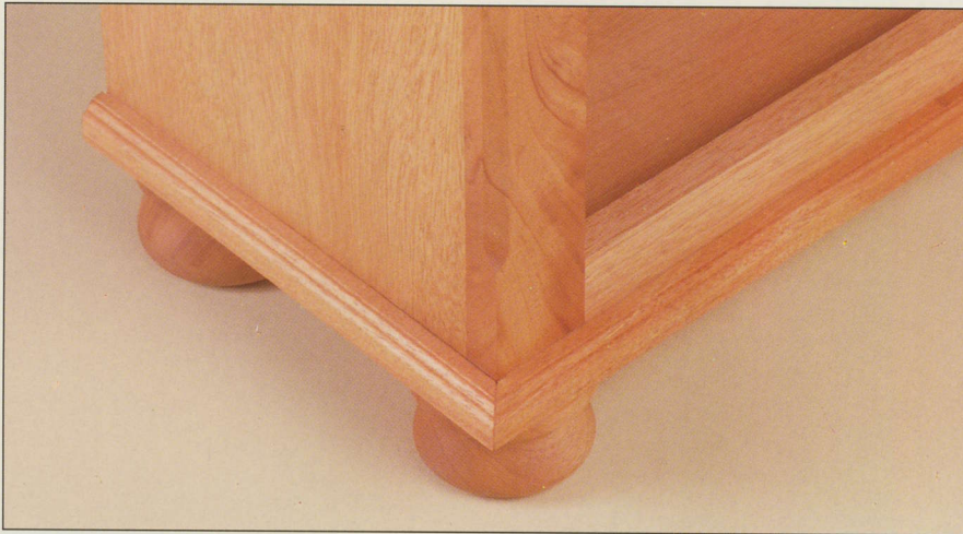
Base molding and feet add a finishing touch to a bookcase. The molding can be routed to match the crown molding or the surrounding trim in the room.
