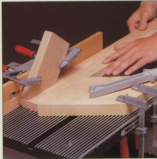
A length of molding is shaped on a router table. Fixed to the base or the top of the carcass, molding provides a classic touch to a bookcase.
